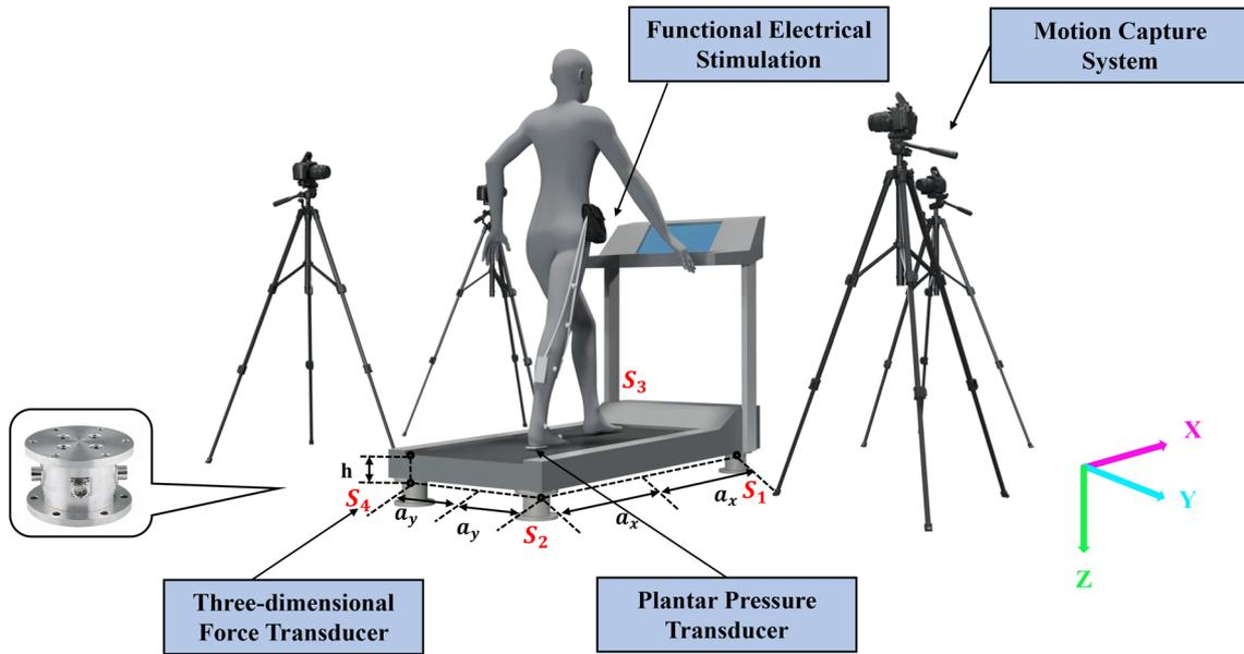
**Fig. 1** The structure diagram of the adaptive FES system. The arrows indicate the positive directions of the three-dimensional force sensors, while  $S_i$  ( $i = 1, 2, 3, 4$ ) represents the  $i$ -th sensor
